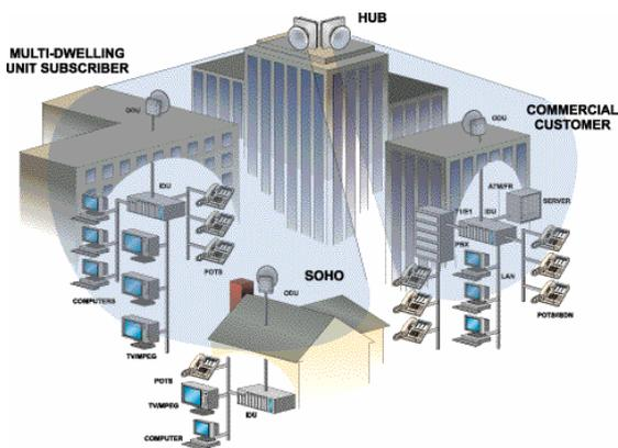
Fig.7. Hughes AIReach 900 system structure
