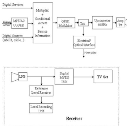
Fig.6. Transmitter and Receiver of the COMMUTE system
