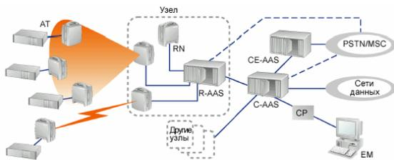
Fig.3. Ericsson Mini-Link™BAS System Structure
