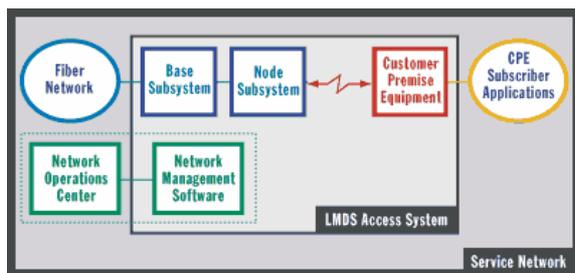
Fig.11. SpectraPoint Model 2200 system
