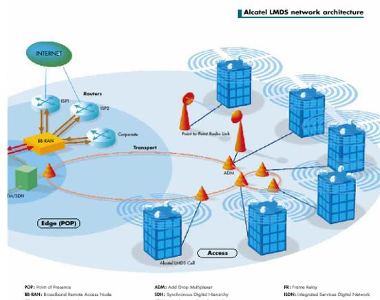
Fig.2. Alcatel LMDS Network Architecture
