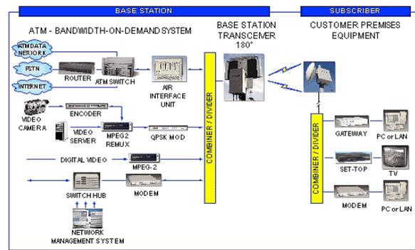
Fig.4. CableAmI system structure
