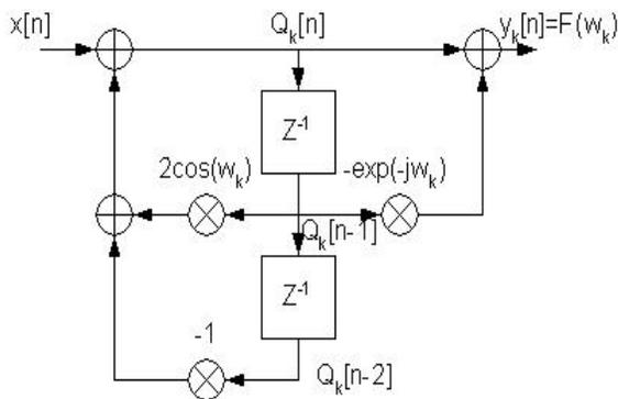
Fig. 2. Block diagram of Goertzel's algorithm
